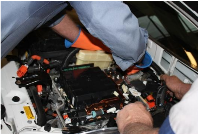
Removing the Inverter
